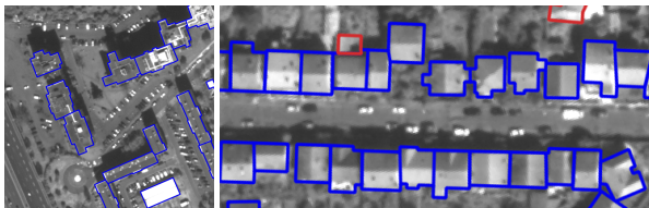
Figure 7. Apartment buildings and their instance annotation provided in the data set (indicated in blue). Red marked objects are not identifiable and excluded from evaluation.
