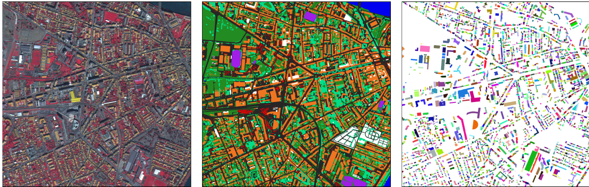
Figure 1. 1 out of 16 tiles of the SemCity Toulouse data set (876 px \times 863 px, area covered \approx 3 km 2 ). Illustrated are the satellite image (near infrared-green-blue), semantic segmentation annotation, and building instance annotation (from left to right).
