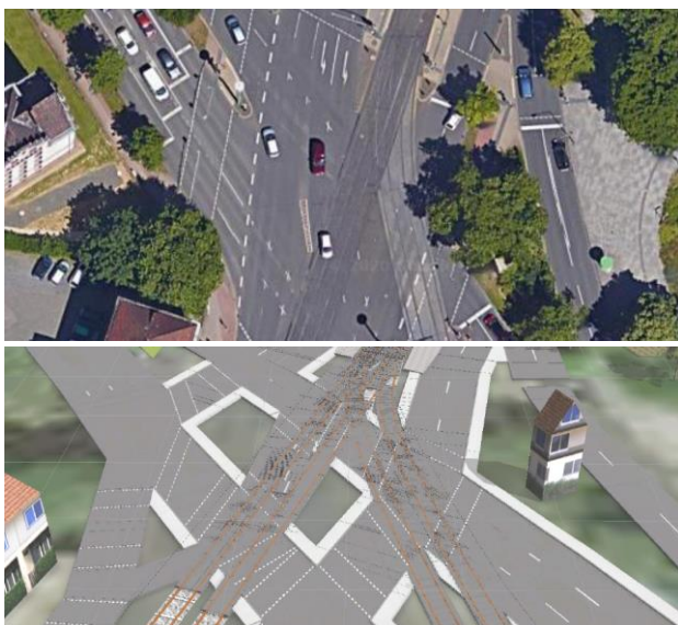
Figure 1. Complex intersection of roads and trams. GoogleEarth (top), model generated with CityEngine (bottom) (Gnatz 2018)
