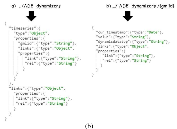
Figure 4. Conceptual model (a) and JSON-based schema (b) of the “dynamizers” main resource
