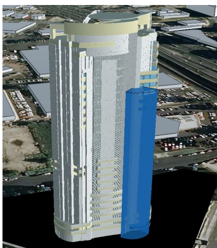
Figure 4. Overlooking regulation in 3D using CSG
