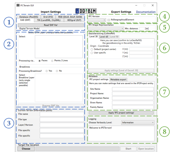
Figure 6. IfcTerrain GUI for simple but configurable conversion of terrain models (DTM) to IFC. (1) input file format selection, (2) format specific import settings, (3) quick input information panel, (4) IFC export version, (5) concept for shape representation, (6) concept for georeferencing, (7) metadata and IfcProject settings (8) logging and verbosity level
