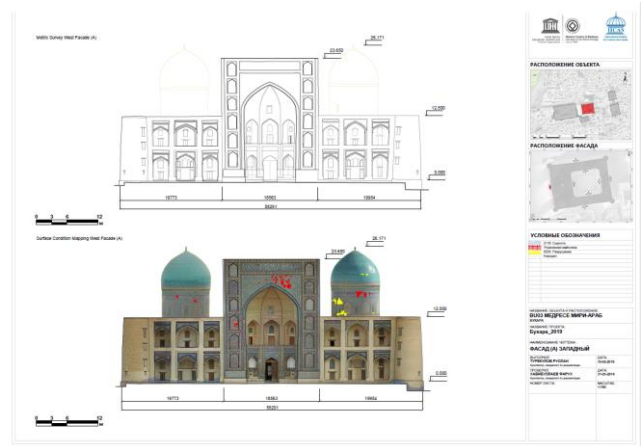
Figure 11. Drawing and orthophoto mapping damages of north Façade of Miri-Arab Madrassah. Source: authors.
