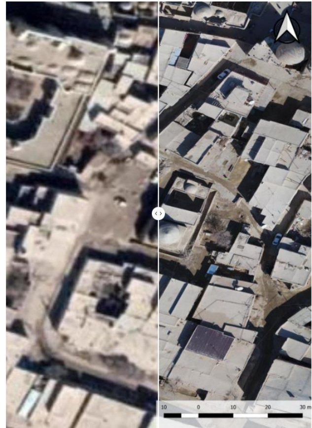
Figure 4. Aerial images. Google Earth (left) and CAAL Orthophoto – UAV flight altitude: 35m (right).
