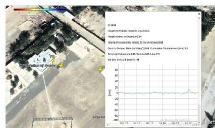
Figure 7. Time series and displacement velocity (in LOS) P1 point are located near the SARAVAN GPS station
