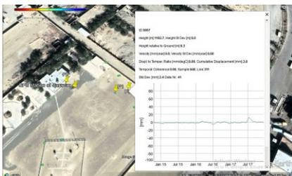
Figure 9. Time series and displacement velocity (in LOS) P3 point are located near the SARAVAN GPS station
