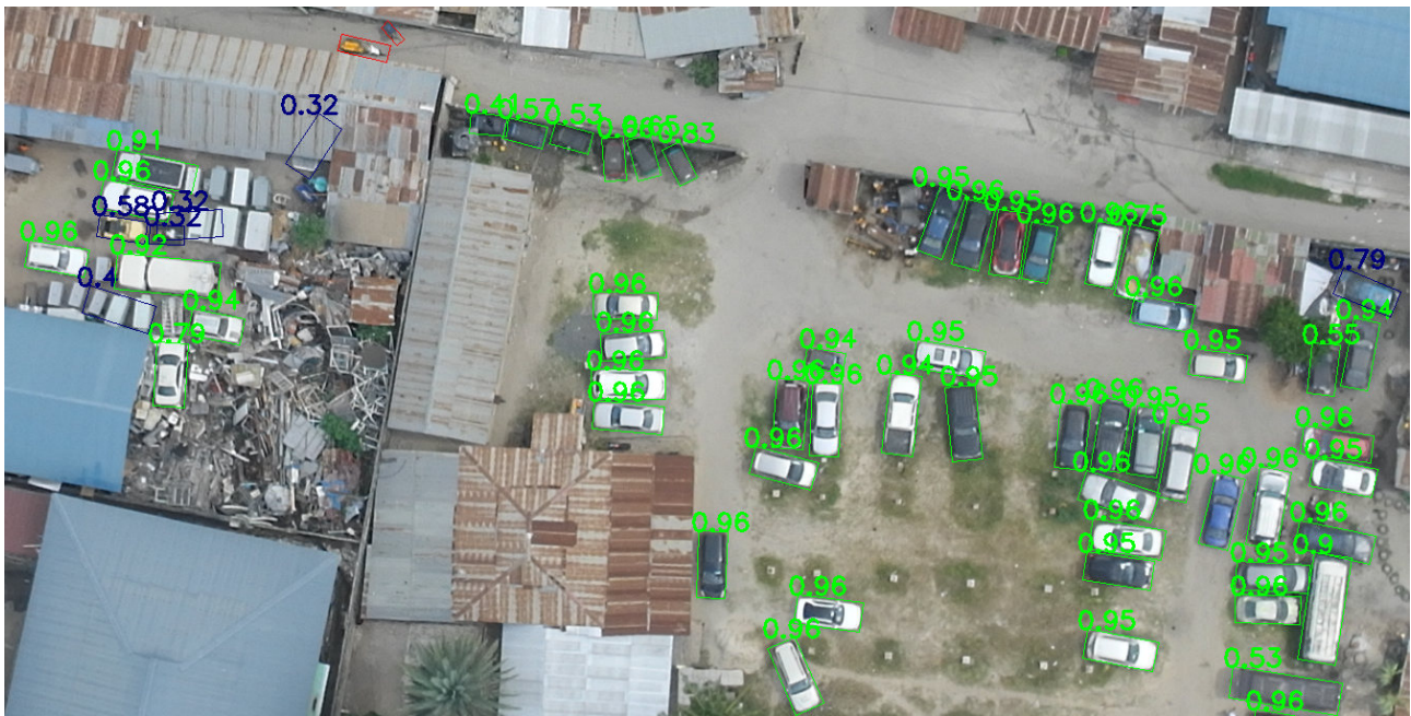
Figure 5. Confusion plot of DINO_{OBB} on a test image crop from XWHEEL. The confidence threshold is set to 0.3 and the IoU threshold, overlap with the ground truth for a detection to count as a TP, is set to 50%. The different entries are color coded: ■ TP, ■ FP, ■ FN, ■ False Class. Additionally, the confidence scores of the inference are plotted next to each detection.
