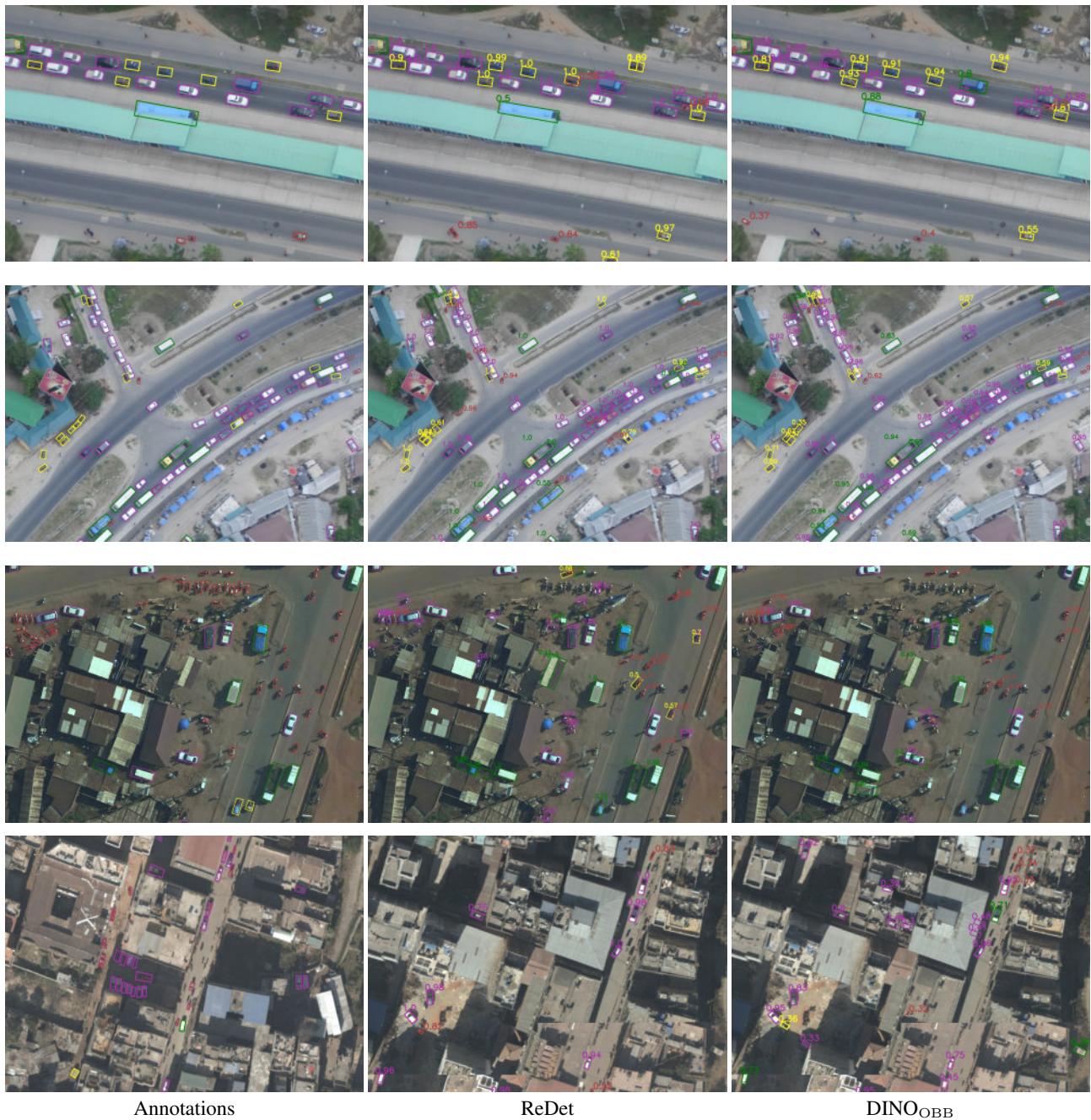
Figure 4. Results of ReDet and DINO OBB on Dar es Salaam (first two rows), Kampala (third row), and Kathmandu (fourth row) for ■ l4w, ■ s4w, ■ m3w, ■ 2w classes. Additionally, the confidence scores of the inference are plotted next to each detection.
