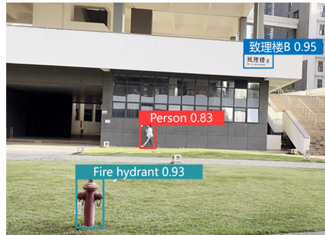
Figure 3. Extracting environmental semantic information through target recognition and OCR
