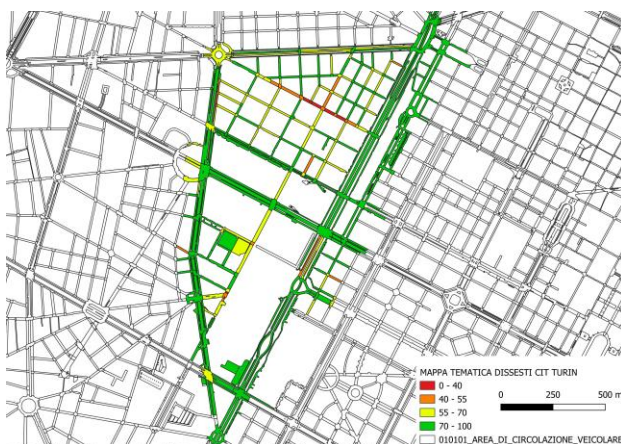
Figure 16. Thematic mapping of the municipal information layer integrating the data extracted from pavement condition analysis, limited to the area surveyed with the MMS
