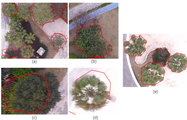
Figure 3. Detectree2 canopy boundary detection effect.(a) and (b) There are undetected canopy boundaries.(c) and (d) Detected canopy boundary position offset.(e) The canopy boundary detection is correct.
