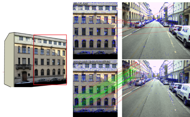
Figure 1. Classical (top) vs learnable (bottom) feature matching methods on a 3D building model's (left) texture image (middle, red rectangle) to mobile mapping image (right) with green lines connecting inlier matches (<30 px projection error).
