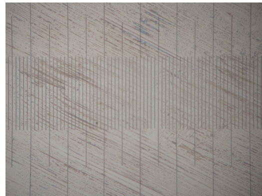
Figure 1. Microscopic photo of ruler used to evaluate the distortion.
