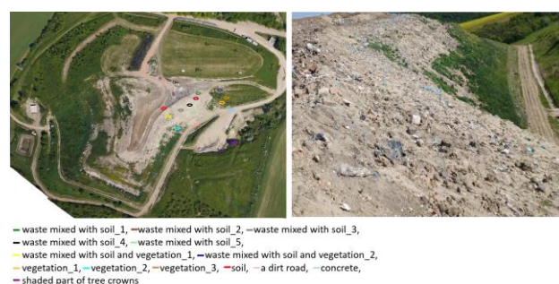
Figure 5. UAV orthophoto of Klobouky u Brna landfill with highlighted zones to analyse apparent temperature from UAV TIR (right). Photograph of the southeast landfill slope where the zones are located (left).
