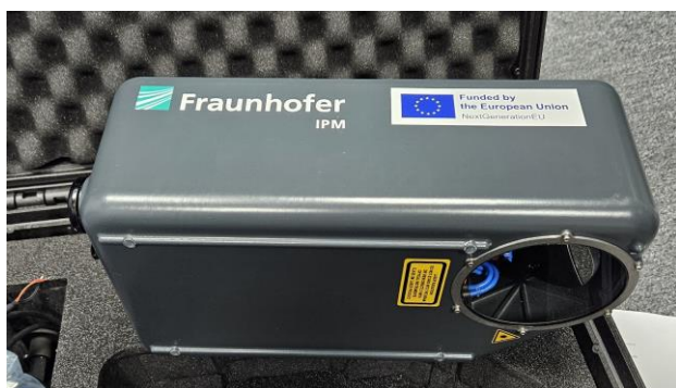
Figure 1. The ABS on its side on top of the transport box. The rotating mirror is visible through the round window.
