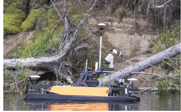
Figure 1. Picture of the USV equipped with the rotating platform and Riegl's miniVUX-1UAV. Photo by Ville Kankare.
