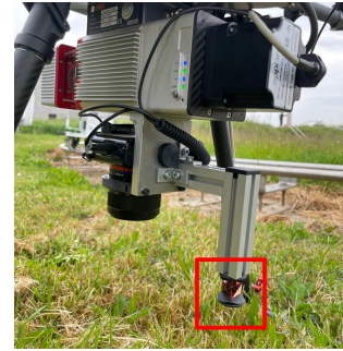
Figure 3. Sensor setup with the additional Leica 360° prism.
