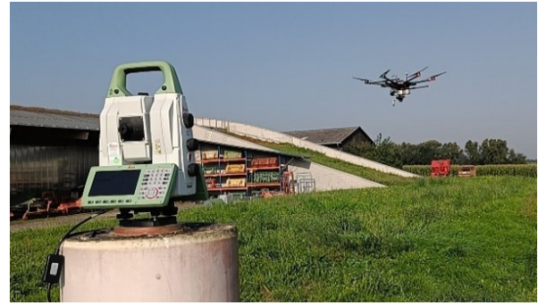
Figure 5. Leica TS 60 (left), on a precisely coordinated pillar tracking the UAV(right).
