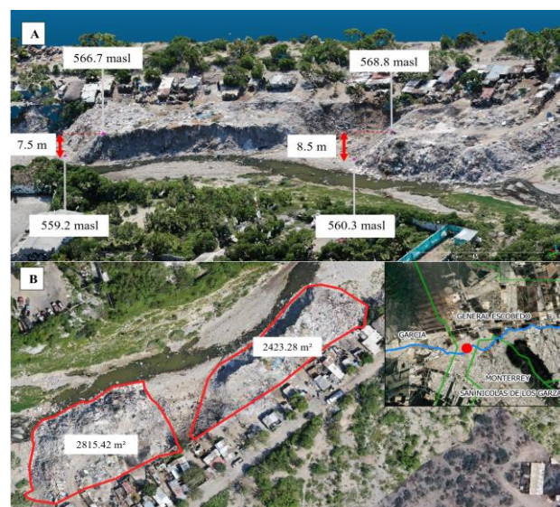
Fig. 6. Accumulations of solid waste on the river, showing A) Heights and elevations, and B) Surface area of the waste.
