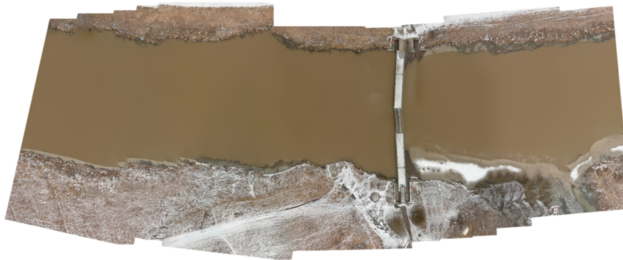
Figure 11. Ortho-mosaic generated from Sixty frames captured during out-door UAV flight.
