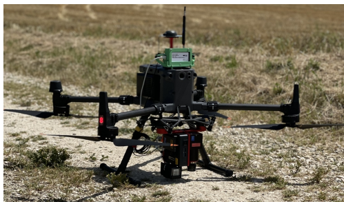
Figure 2. Pika-L HS camera mounted on a DJI M350
