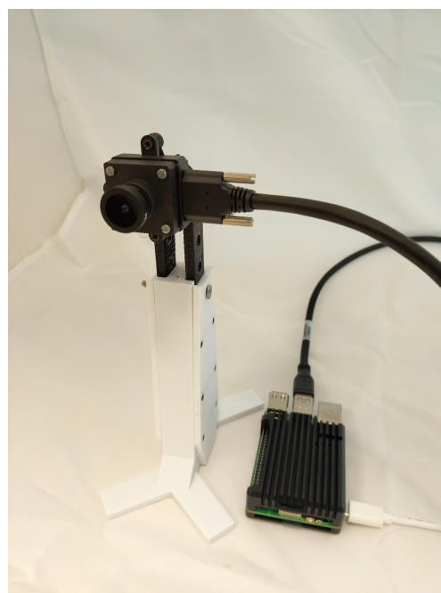
Figure 1. Hardware aspects of the framework: Raspberry Pi 5 single-board computer connected to a Basler RGB machine vision camera with Evetar lens.
