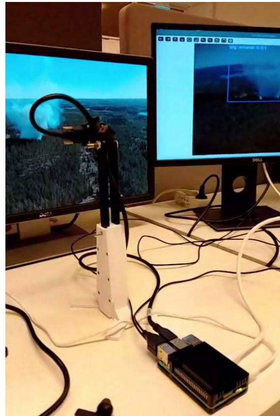
Figure 4. Edge device setup. Left: A machine vision camera acquires a screen that shows UAV-collected video material from the Boreal Forest Fire dataset. Right: The second screen shows the results, where the detected wildfire is surrounded with a blue bounding box, and the prediction confidence is printed on the screen. The Raspberry Pi computer, that processes all tasks, is at the bottom of the image.
