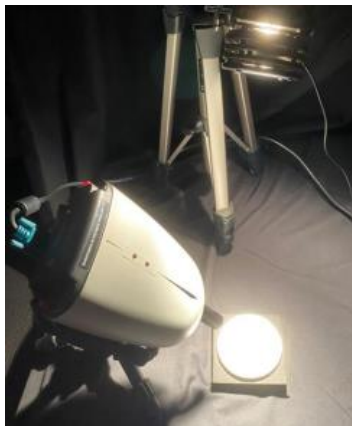
Figure 3. FieldSpec® UV/NIR Handheld spectroradiometer measuring a highly diffuse reflectance calibration plate in a laboratory, with the aid of a halogen light.
