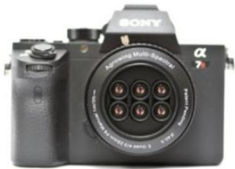
Figure 4. Sony Alpha 7Riv Sextuple camera ( Agrowing camera), with six heads.
