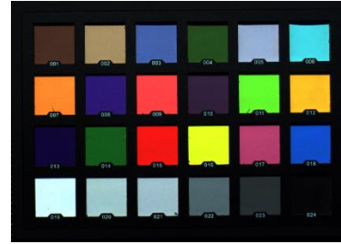
Figure 7. Colorimetric plate with 24 colors which has been tested for radiometric calibration of images.
