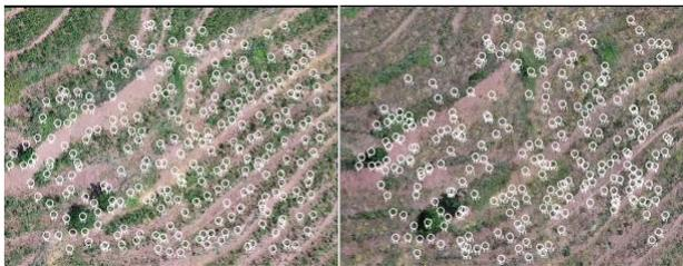
**Figure 11.** Corresponding image points based on image matching
