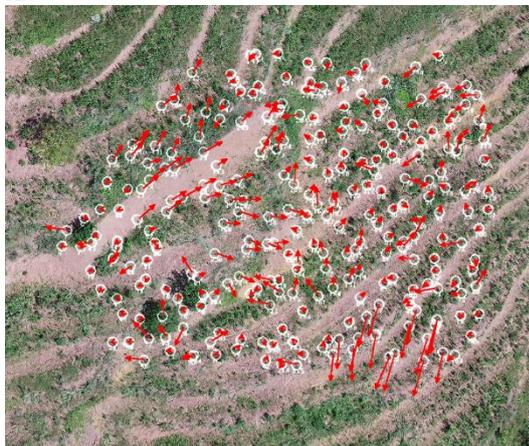
**Figure 12.** Displacement of deformation trend.
