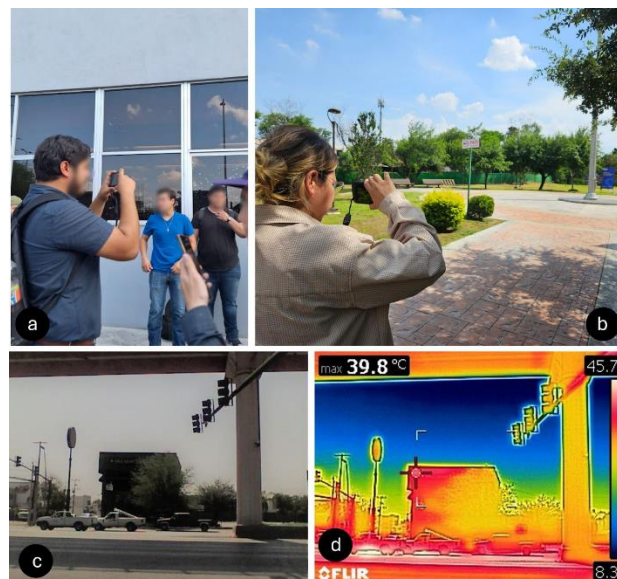
Figure 6. Geomatics students used a thermal sensor in a microscale capture, a) testing the sensor over various materials, b) in urban green areas, c) RGB visible light sensor and d) a thermal image.
