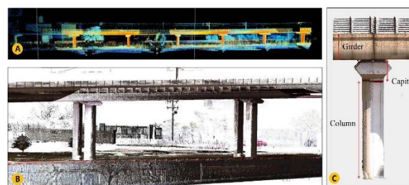
Figure 4. A first view of the aligned structure. (A) The aligned point cloud displayed with intensities and (B) The aligned pcL merged with the RGB
