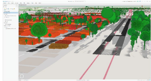
Figure 11: Integrated voxel data imported as a point cloud layer into ArcGIS Pro
