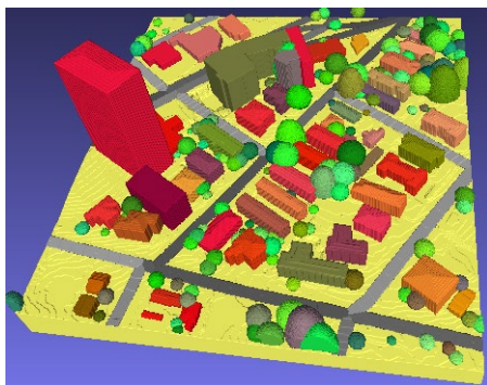
Figure 7: Final integrated 3D scene in L1 (40cm voxel resolution)
