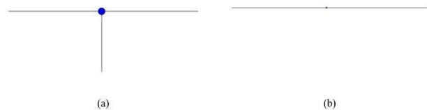
Figure 7. Street intersection node identification and pre-processing: (a) node at the shared location of three segments; (b) no node at the intersection of two segments.
