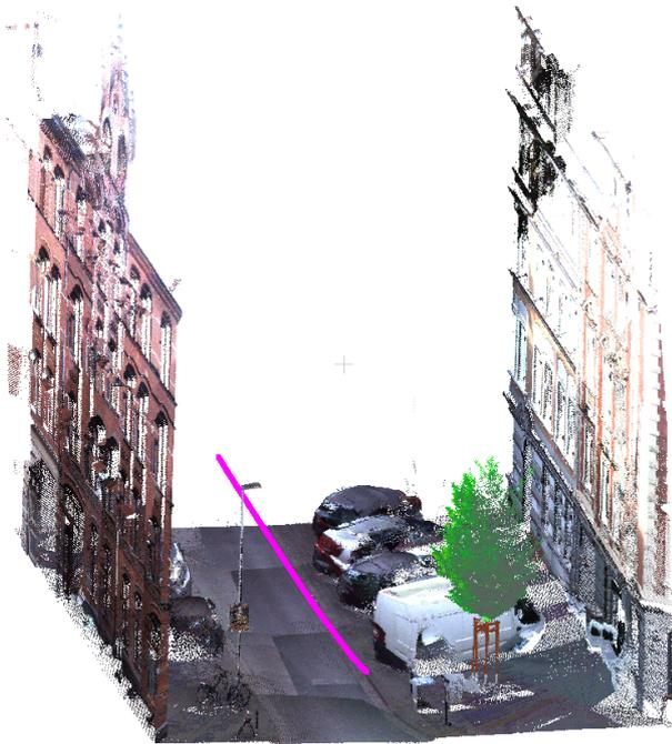
Figure 1. The point cloud measured by the Mobile Mapping System, with the trajectory of the sensor movement, represented by the magenta line.
