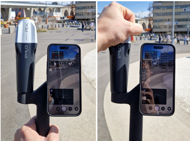
Figure 2. iPhone with PIX4Dcatch connected to the RTK device: Emlid RX (left). Covering the antenna (right) simulates the loss of RTK fix in the same scene with measured check points.
