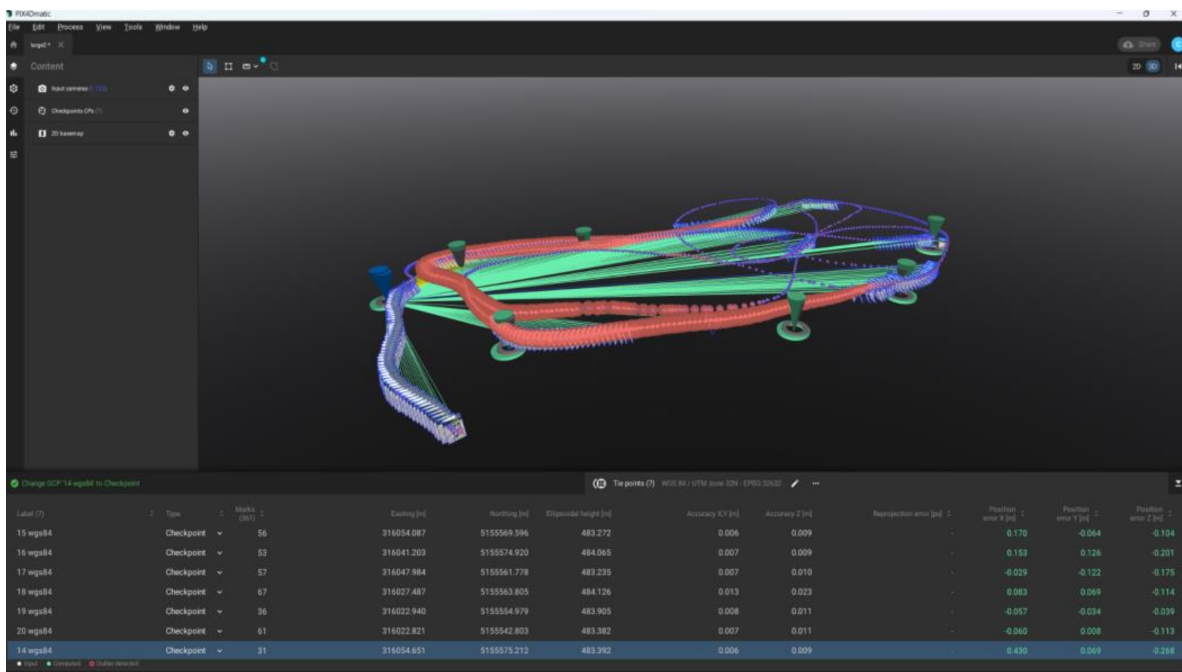
Figure 8. Importing and marking Checkpoints inside PIX4Dmatic. Dataset 2 with partial coverage of the antenna and higher uncertainty of the image positions (visible here as red ellipsoids).
