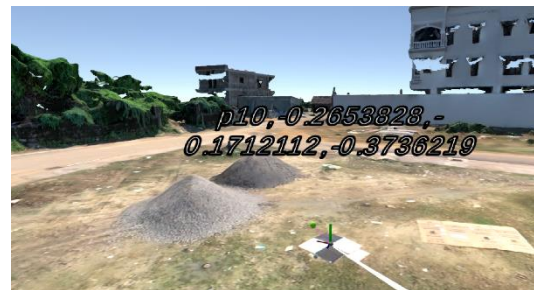
Figure 9. The labels on top of the Observed points display the deviation values along the x, y, and z-axis.
