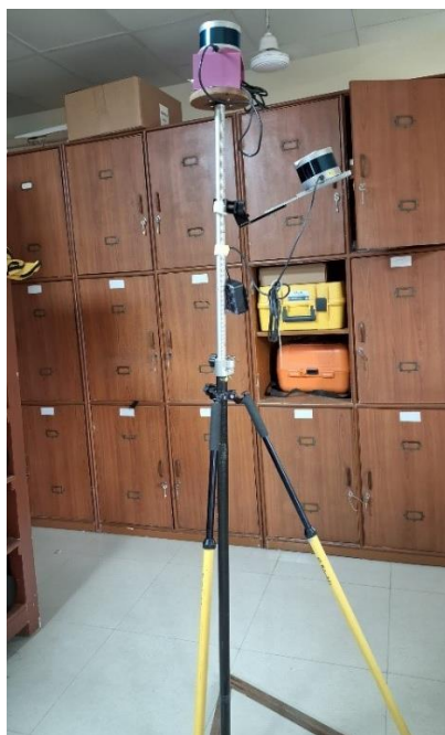
Figure 1. Experimental Setup for two VLP16 sensor.
