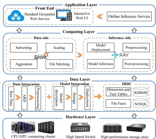
Figure 3. Implementation architecture of the system.
