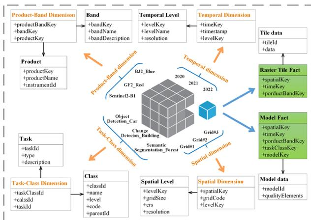
Figure 2. A cube approach to accommodate GeoAI models.
