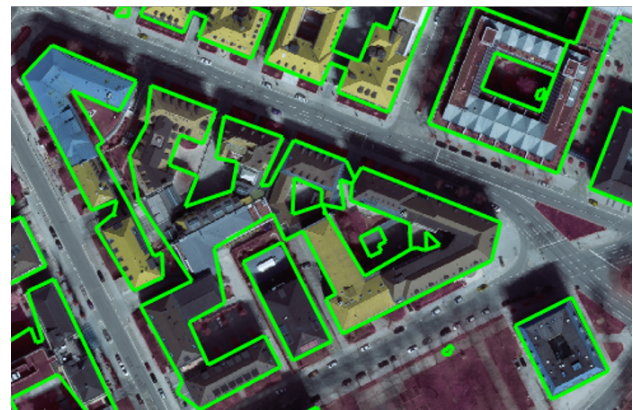
Figure 6. Example on building outlining from Figure 5 using the IOSB method, with too high (top) and regular, slightly too low (bottom) value for \eta .
