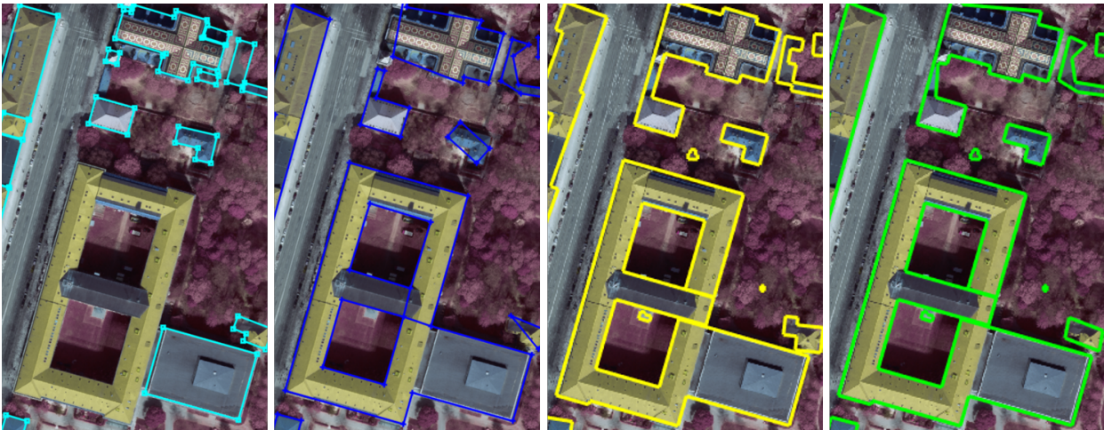
Figure 3. Extended building with inner courtyard. Cyan, blue, yellow, and green color: Mapflow, Al-Muthanna, IOSB results (too high value of \eta , and a regular \eta ).
