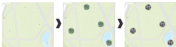
Figure 3. Polygon "Stamp" process from points set by the user to duplicated polygons and their rasterization.
