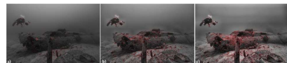
Figure 15. Comparison of SIFT keypoints vs CLAHE parameters on a single image from the B17 " Black Jack " Aircraft wreck (1943). (a) original image, (b) recommended parameters, and (c) default parameters.
