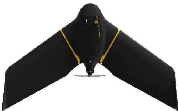
Figure4. Sensefly eBee X fixed-wing drone
