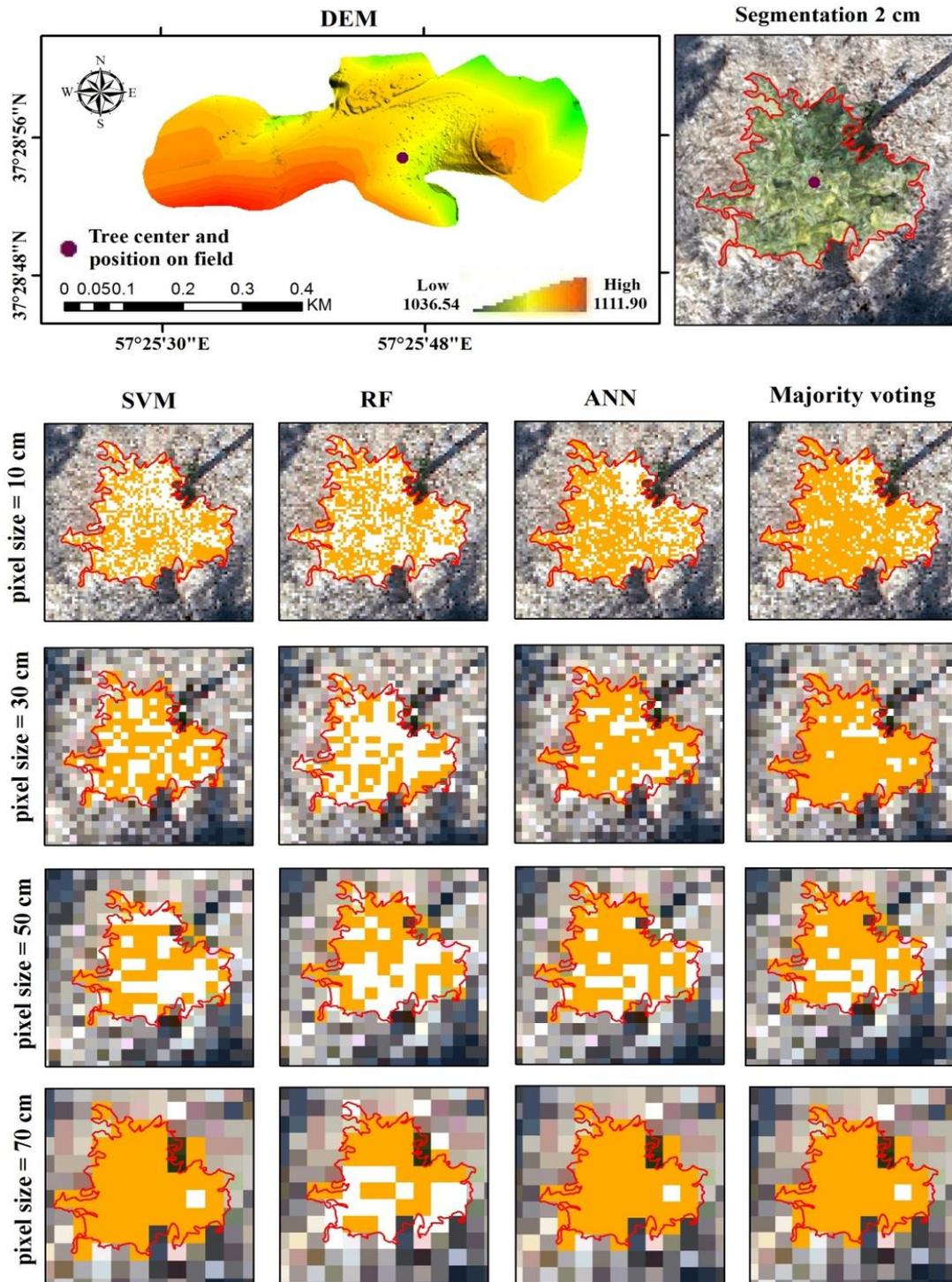
**Figure 3.** A part of classification results of SVM (Support vector machine), RF (Random forest) and ANN (Artificial neural network) used to delineate *Pinus eldarica* tree crowns (red polygons) on UAV orthoimages with pixel sizes of 10, 30, 50, and 70 cm. The red polygon is the true crown boundary obtained from segmentation of the 2-cm resolution orthoimage overlaid on the orthoimages with different pixel sizes for visual interpretation.
