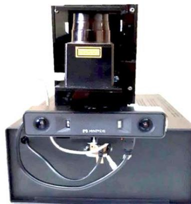
Figure 4. The integrated sensor is composed of a 2D LRF, a stereo camera, and a servomotor
