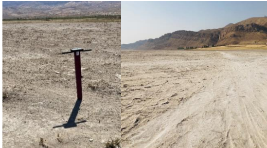
Figure 2. Top photo, TDR 350 device for In-situ data collection, Bottom photo, a general view of the study area.
