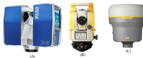
Figure 2. Instruments used for the experiment (A) TLS, (B) Total station (TS), (C) GNSS receiver.
