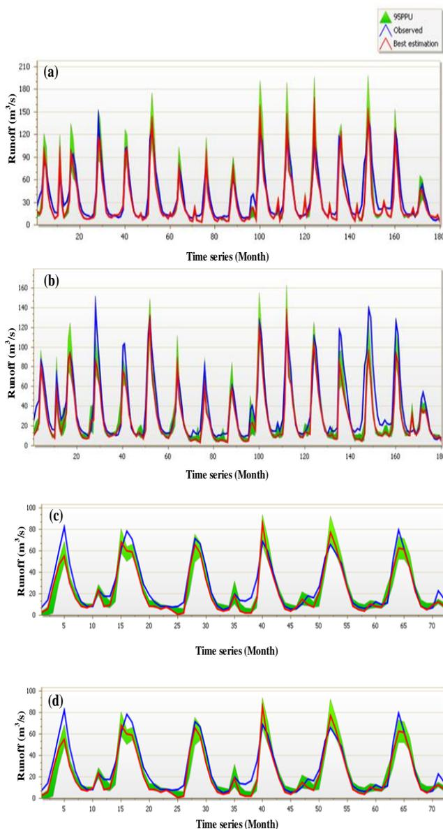
**Figure 4.** Discharge calibration results for the period of 1994–2008 using (a) GRGs dataset and (b) SPPs dataset. Discharge validation results for the period of 2009–2015 using (c) GRGs dataset and (d) SPPs dataset.
