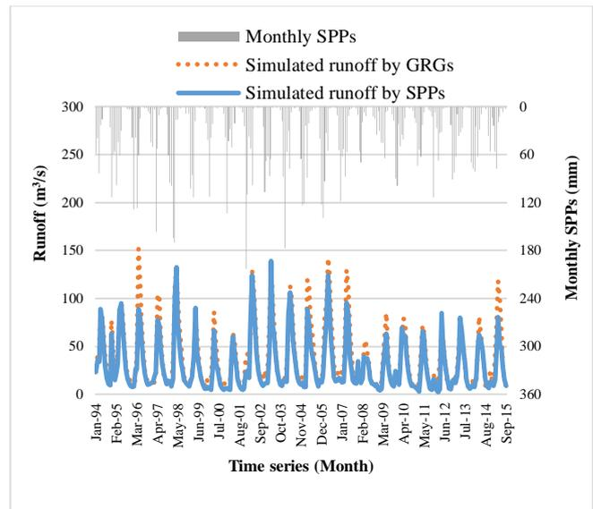
**Figure 5.** Time series of the best runoff simulated by the SWAT model using GRGs and SPPs datasets, and PERSIANN-CDR total monthly precipitation over the period of 1994-2015.
