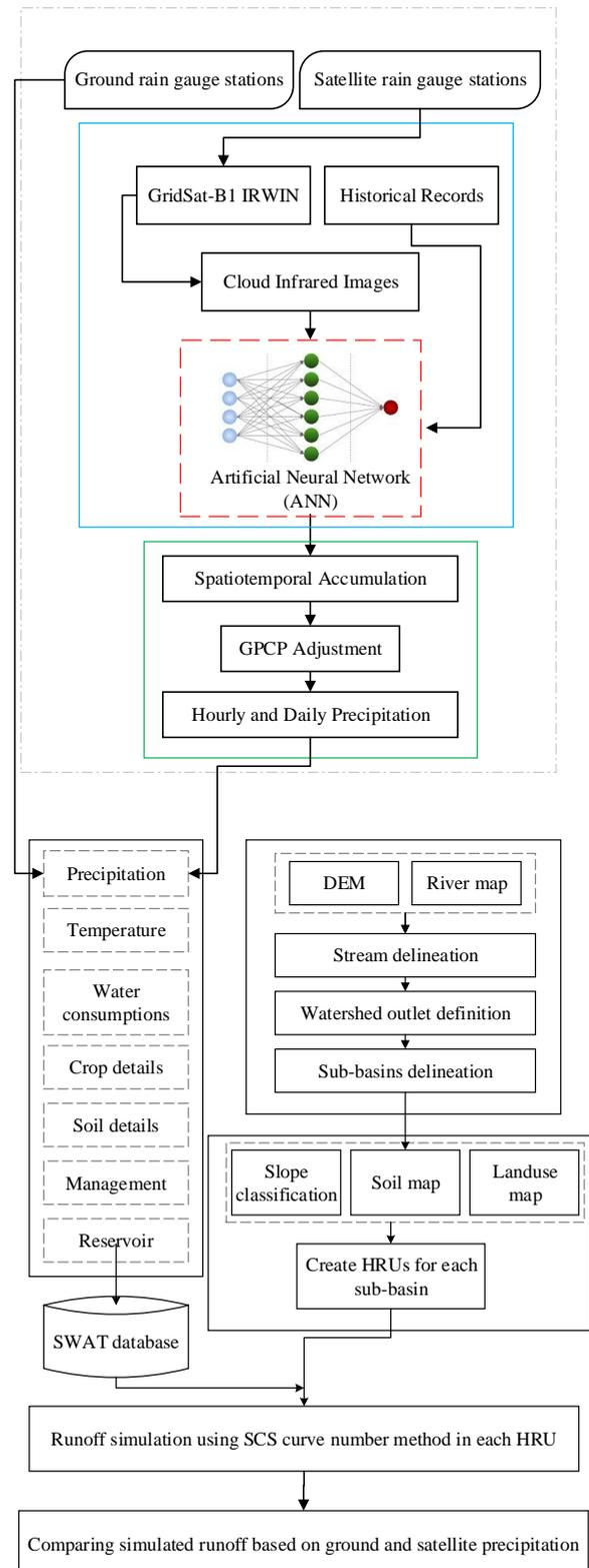
**Figure 2.** Flowchart of the proposed method for comparing simulated runoff based on SPPs and GRGs data.
