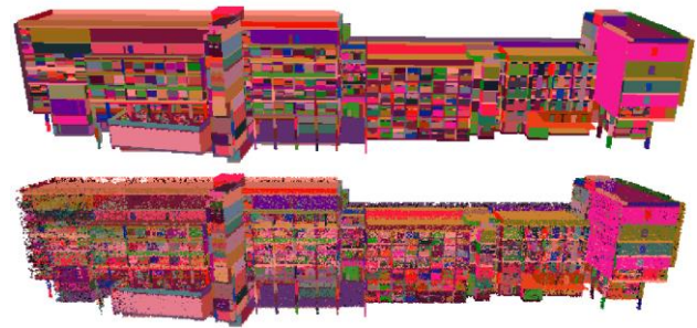
Figure 7. Rendering voxels as point clouds; upper image shows all voxels as points; lower image shows some randomly culled voxels based on the distance to a camera
