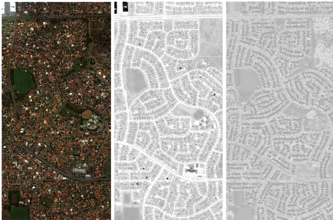
Figure 2. Orthophoto (left), measured (middle) and simulated temperatures (right) in white-hot representation.
