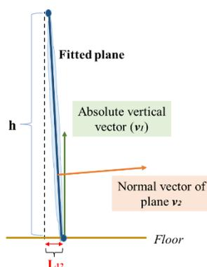
**Figure 3.** Verticality deviation computation.
