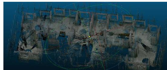
**Figure 4.** Collected point cloud data of the selected case using BLK 360.
