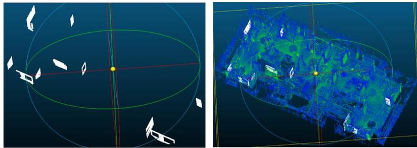
**Figure 7.** Identified faulty wall planes (left) and their locations in the floor (right).
