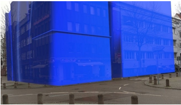
Figure 5. Alignment of the 3D building model occlusion mask with real environment. Rendered in blue color for better visualization.
