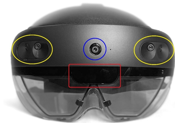
Figure 3. HoloLens 2.0 camera configuration. (yellow) Grayscale tracking cameras. (Red) ToF camera. (Blue) RGB camera.
