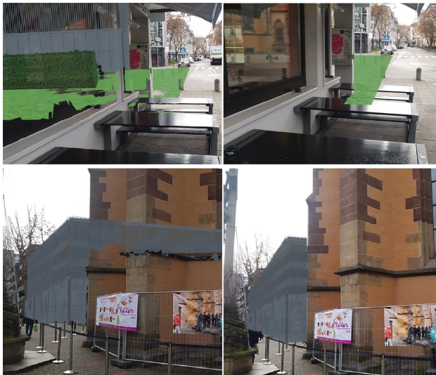
Figure 8. Comparison between occlusion screening based on (left) the Spatial Map and (right) the 3D building model.
