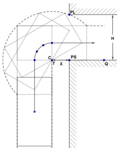
Figure 9. The trajectory of RRB when  $X \geq \sqrt{L^2 + W^2 - H^2}$ .
