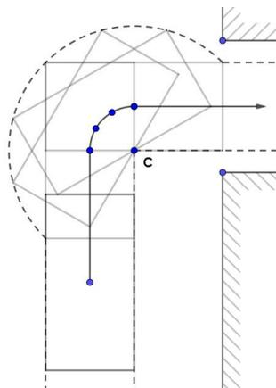
Figure 5. The trajectory and required space of RRB with a rotation centre. The line with the centre of RRB is the trajectory and the space between the two dash lines is the required space.
