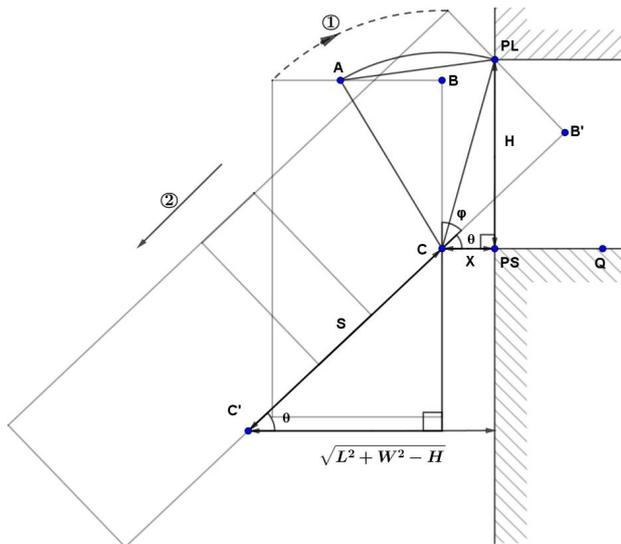
Figure 11. The illustration of calculation process of  $\theta$ .
