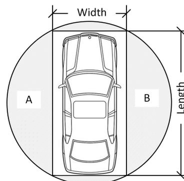
Figure 1. Comparison of modelling a rigid-body as its smallest circumcircle and a rectangle with length and width.
