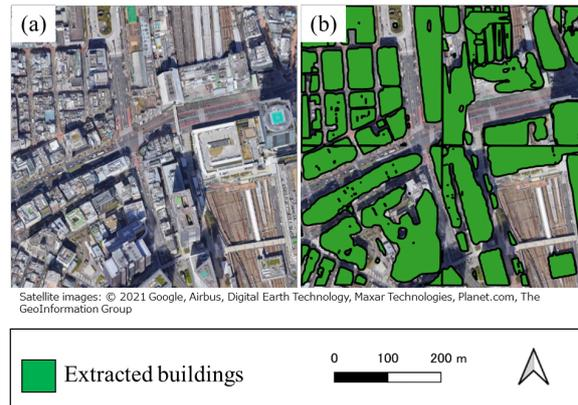
**Figure 2.** Example of building detection results (Vicinity of Shinjuku Terminal, Shinjuku-ku)
