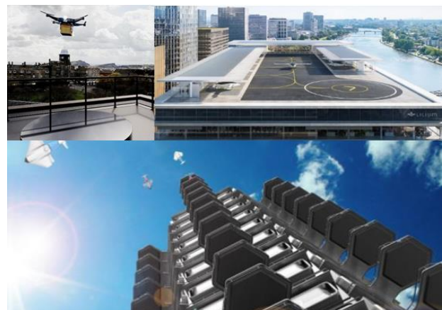
Figure 14. Design plans for Urban-Verti-Ports: a) (left) on a terrace for small-delivery drones, b) (left) on a roof for larger-passenger UAVs, and, c) (down) on the balcony extensions of a building for private/personal vehicles.
