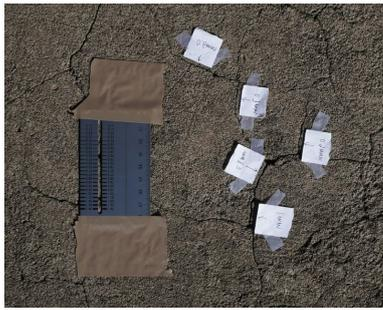
**Figure 11.** Crack measuring gauge and labeled cracks.
