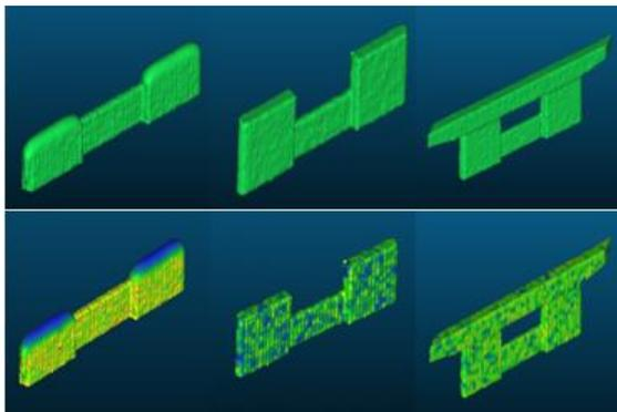
**Figure 9.** Poisson surface reconstruction results and their quality heat map for 3 cases of Pier 1.
