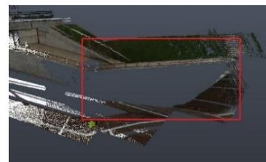
Figure 4. The occlusion of point cloud on the retaining wall.
