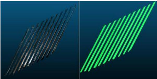
**Figure 11.** The as-built point cloud for eleven girders in Span 1 and their 2D polygon fitting results.
