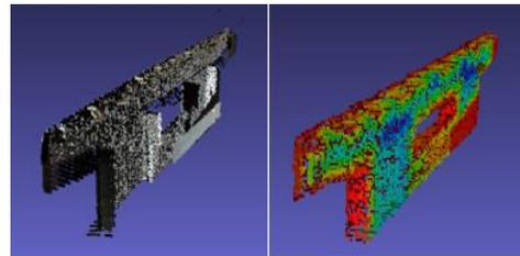
**Figure 10.** The occlusion on the surface of pier (Left) and the quality heat map after Hausdorff distance simplification (Right).
