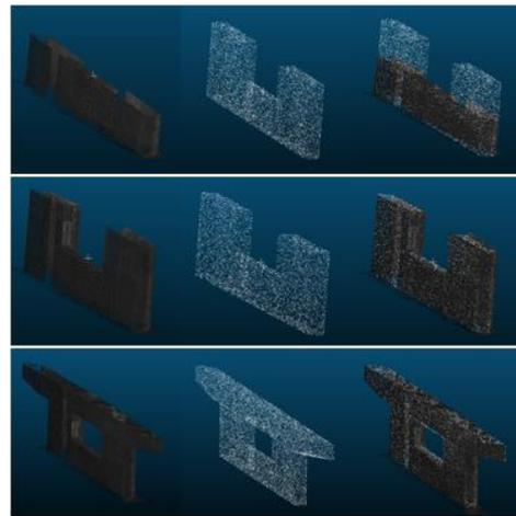
**Figure 7.** The as-built point cloud, virtual point cloud and registration results for case 1, 2 and 3 of Pier 1 (Left to right, top to bottom respectively).
