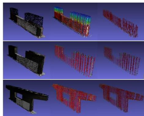
**Figure 8.** The registration results, Hausdorff distance sampling heat map and simpling results for 3 cases of Pier 1 (Left to right, top to bottom respectively).
