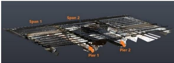
**Figure 5.** An overview of the Kapooka bridge (white and shadow point cloud are from two different laser scanners).
